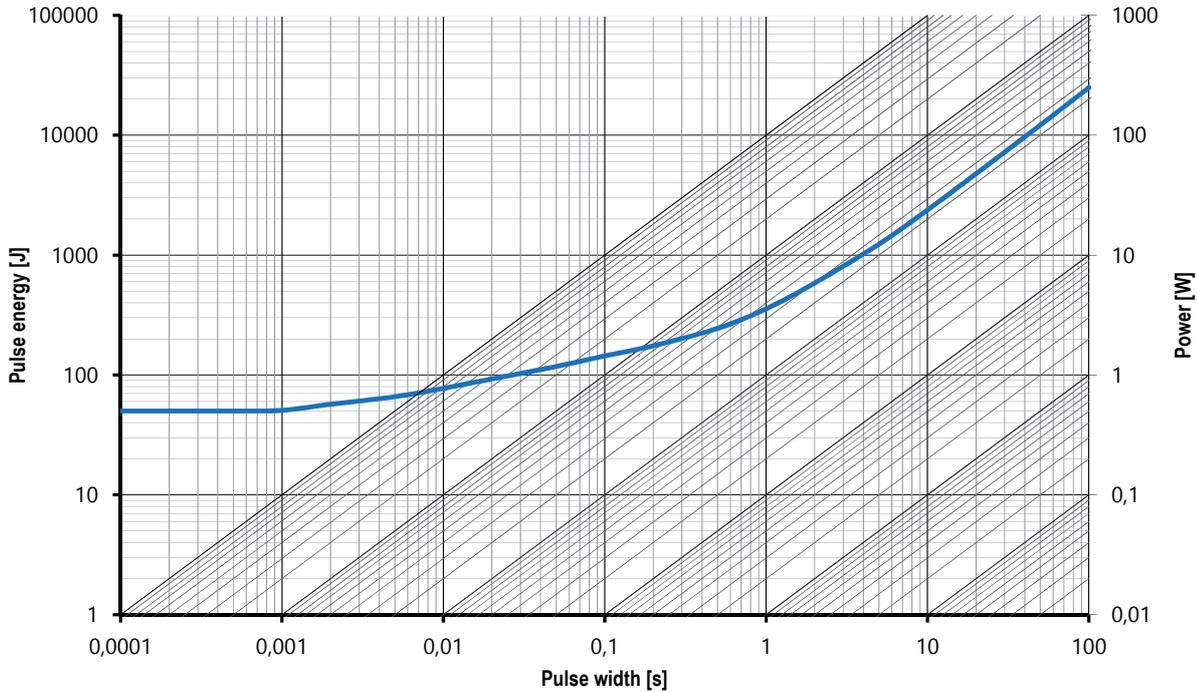
This curve is only valid for the resistance value R001. The shape of the curve will be different for other resistance values. Therefore a separate qualification should be made for pulse power close to the above curve.
